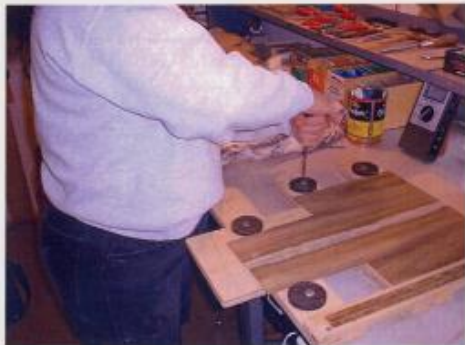
The back plates are glued together in a joining jig.
