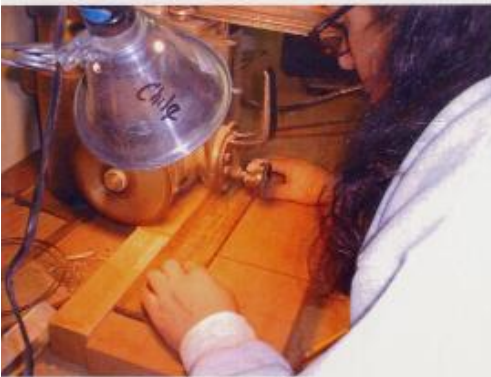
Slotting the fret plate with a radial-arm saw
