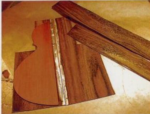
Thinned plates of Acacia wood are sized and joined for the back and sides of the instrument
