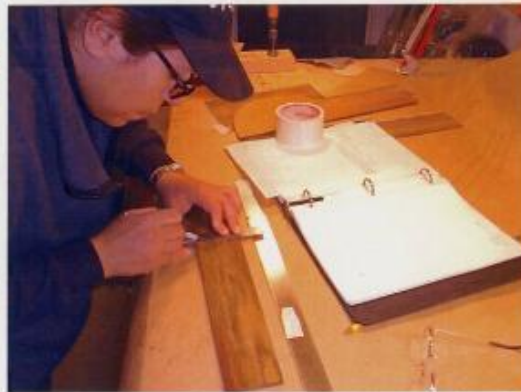
Measuring the fret intervals according to the fretting formula.
