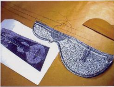
A full-size half- template is derived from a blowup of a 1924 photograph of Heriberto Torres' 8-string cuatro
